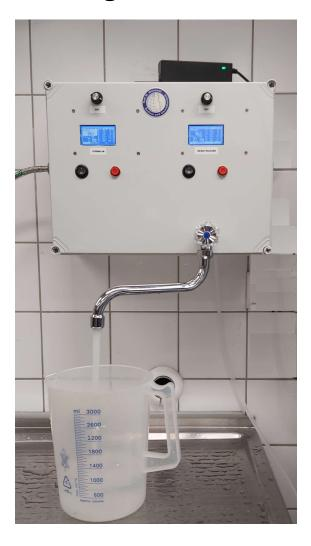
Connection to an in-house ultrapure water line or normal water pipe. Formalin with 38% is aspirated from a canister via a pump and mixed with the ultrapure water according to your according to your requirements.
