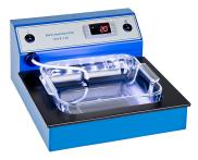
Square water bath with illumination Digital temperature display and control. Water bath removable. Only the glass pan is transported for water change. Cleaning the glass pan in the dishwasher. Side shelf for slides. Water bath: 210 x 210mm Height 55mm Overall dimensions: W310 x L355 x H170mm Temperature max. 60 ° C Power ratings: 230V / 50Hz / 200W Article No. WBQL
